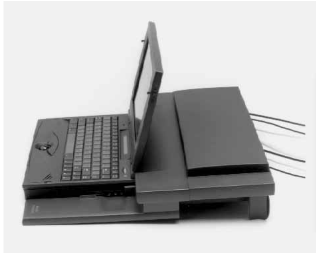
Fig. 4. HP OmniBook 5000 computer in docking station.
