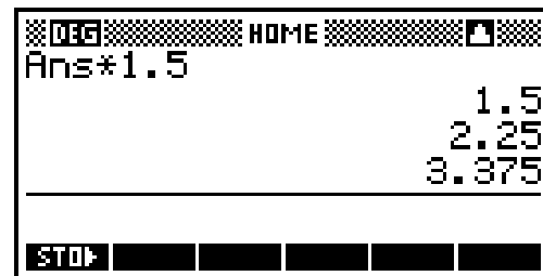
Fig. 28. If the user presses ENTER without input, the previous input is repeated. This saves keystrokes for iterative operations.
